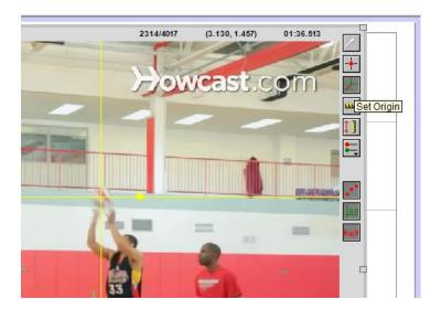
10. This step is not essential, although it does affect the kinematic models you generate. Here, I set the origin of my Cartesian coordinate system. I've chosen to do so in the center of the ball, in the frame where the ball has just begun its free fall motion. To set the origin, simply click on the Set Origin button on the side of the window, then click in the video where you wish to place your origin.
